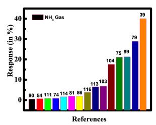
Fig. 11 Gas response of NH<sub>3</sub> gas with Ti<sub>3</sub>C<sub>2</sub>T<sub>x</sub> MXene-based gas sensors.
