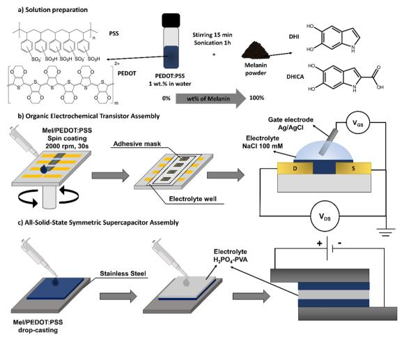
Fig. 1 (a) Preparation of the Mel/PEDOT:PSS OMIEC blend at different concentrations and chemical structures of PEDOT:PSS and Mel subunits (DHI and DHICA). Assembly steps of (b) OECTs and (c) all-solid-state symmetric SuperCaps.
