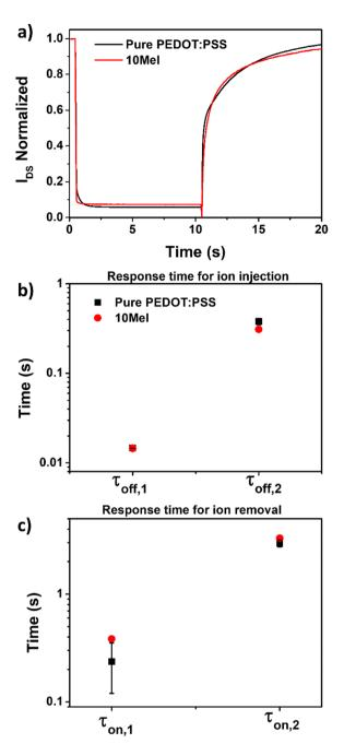
Fig. 7 Response time of OECTs. (a) Normalized  $I_{\rm DS}$ -time curve for OECTs employing 10 Mel and pure PEDOT:PSS films upon application of a single positive  $V_{\rm GS}$  bias +0.8 V (pulse width = 10 s) at fixed  $V_{\rm DS}$  = -0.6 V, and  $V_{\rm GS}$  = 0 V. Corresponding time constants ( $\tau$ ) for the (b)  $I_{\rm DS}$  decay and (c)  $I_{\rm DS}$  growth using a double exponential function.
