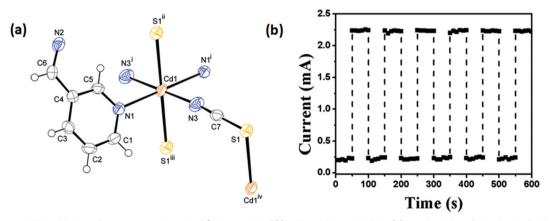
Fig. 3 (a) A thermal ellipsoid plot of an asymmetric unit of 2 drawn with 50% ellipsoidal probability; (b) conductivity of the device fabricated with 2 at light-on and light-off conditions (bias voltage = 1.0 V and intensity of incident light =  $80 \text{ mW cm}^{-2}$ ). Reproduced with permission from ref. 54. Copyright 2015 Royal Society of Chemistry.
