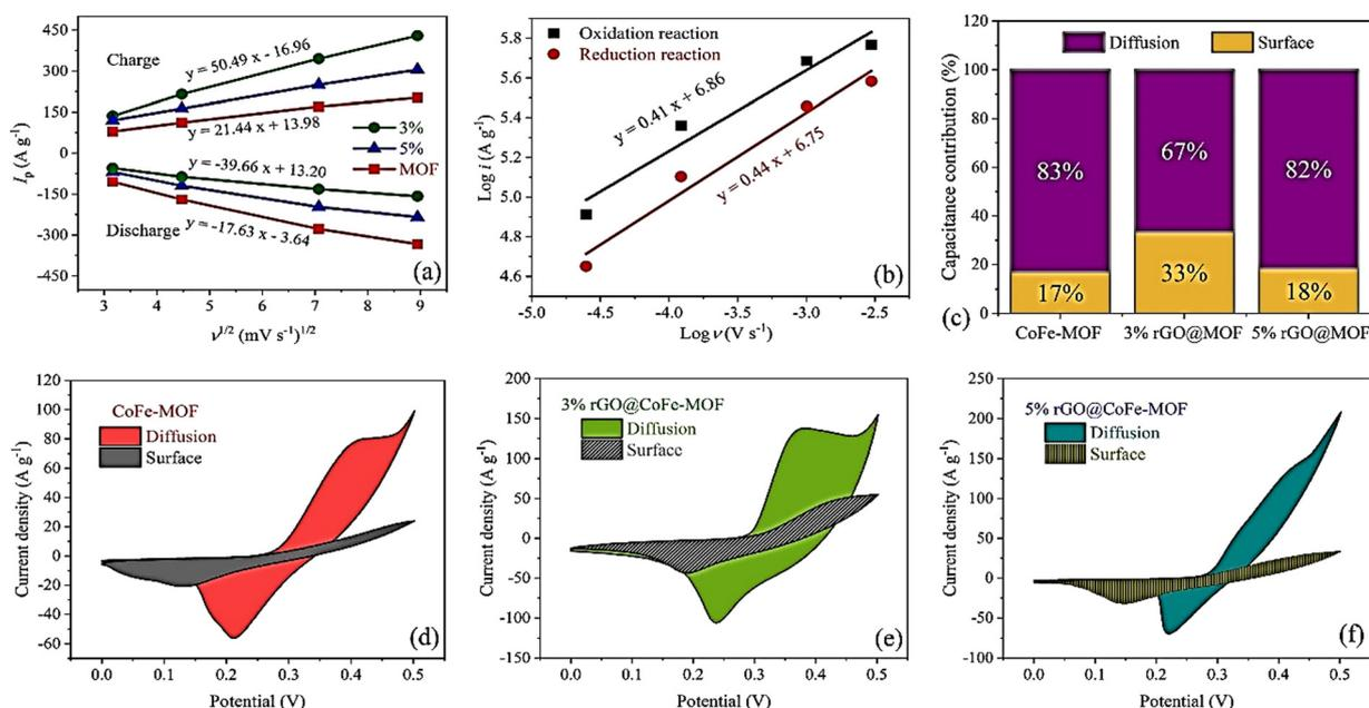
Fig. 18 (a) The curves of the peak current versus the square root of sweep rate (Randles–Sevcik plot). (b) The plots of  $\log i$  versus  $\log v$ . (c) Capacitance contribution for three electrodes, the capacitive contribution of CV curves at 10 mV s<sup>-1</sup> for (d) CoFe-MOF, (e) 3% rGO@CoFe-MOF, and (f) 5% rGO@CoFe-MOF. Reproduced from ref. 173 with permission from Elsevier Ltd, Copyright 2023.
