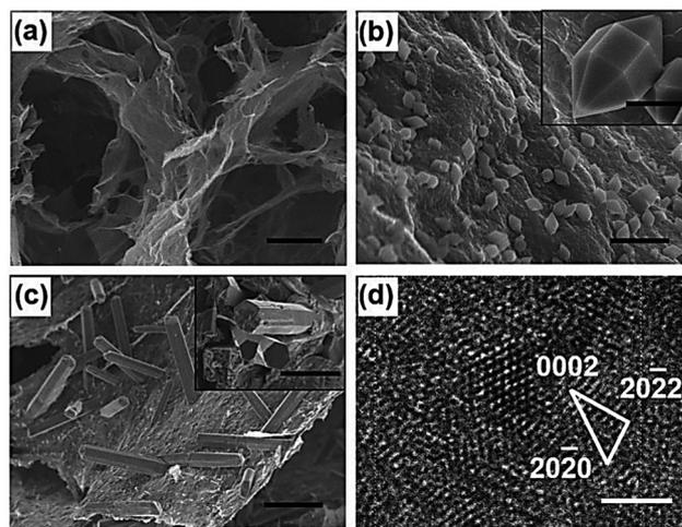
**Fig. 11** SEM and TEM images of GA, GAMOF, and GAMOF(Fe<sup>3+</sup>) composites. (a) SEM image of GA (scale bar: 20  $\mu$ m). (b) Low- (scale bar: 2  $\mu$ m) and high-magnification SEM images (inset; scale bar: 500 nm) of GAMOF. (c) Low- (scale bar: 2  $\mu$ m) and high-magnification SEM images (inset; scale bar: 500 nm) of GAMOF(Fe<sup>3+</sup>). (d) HRTEM image of GAMOF(Fe<sup>3+</sup>) (scale bar: 2 nm). Reproduced from ref. 159 with permission from WILEY-VCH, Copyright 2018.
