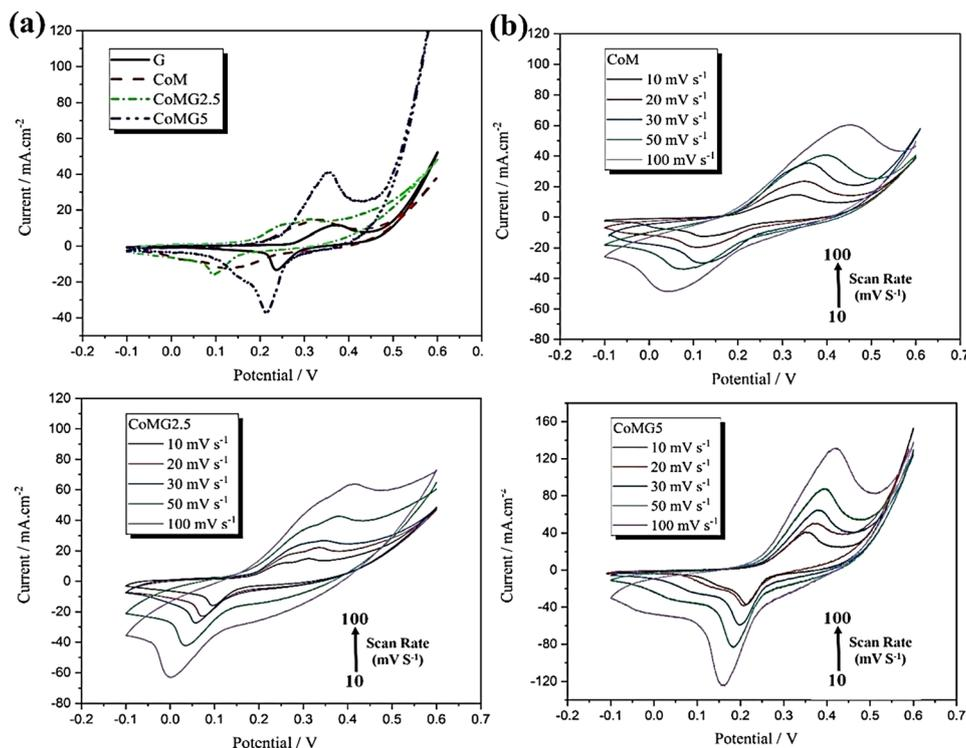
Fig. 6 The CV curves of (a) G, CoM, CoMG2.5, and CoMG5 at a scan rate of  $10 \text{ mV s}^{-1}$ , (b) CoM, (c) CoMG2.5 and (d) CoMG5 electrodes at different scan rates ( $10\text{--}100 \text{ mV s}^{-1}$ ) in  $6 \text{ M KOH}$ . Reproduced from ref. 143 with permission from Elsevier Ltd, Copyright 2021.
