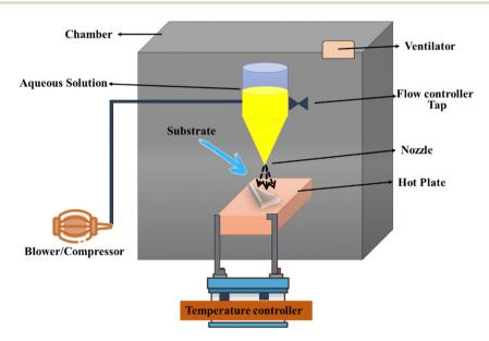
Fig. 7 A complete setup for electrospray pyrolysis.
