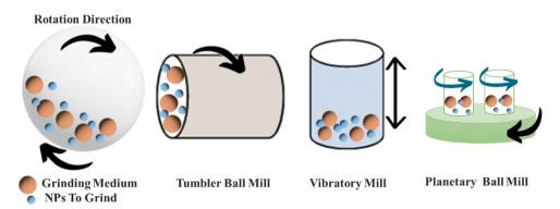
Fig. 5 Different mechanisms for mechanical ball milling
