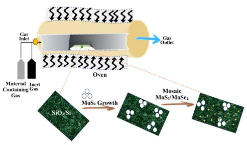
Fig. 13 Synthesis of MoS<sub>2</sub>/MoSe<sub>2</sub> by chemical vapor deposition.
