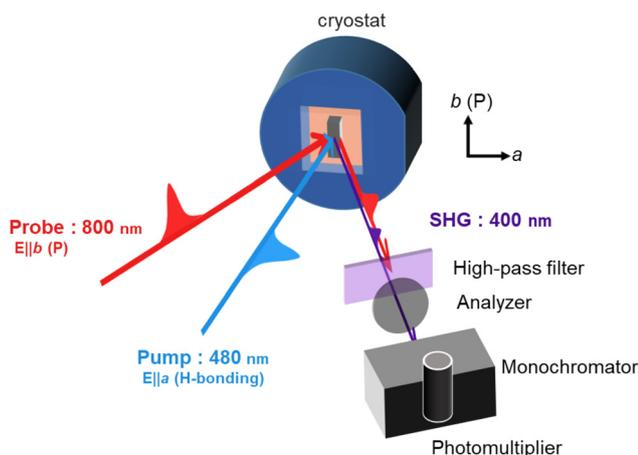
Fig. 2 Experimental setup for the pump-probe SHG measurement. The red and blue pulses denote the probe (800 nm) and pump pulses (480 nm). The Phz-H<sub>2</sub>ca crystal was set in a cryostat and generated SHG pulse was detected by using a photomultiplier through a filter and grating monochromator.
