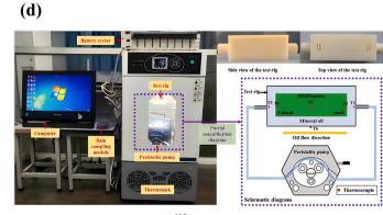
(a) Structure of the BTMS with immersion cooling, 115 (b) schematic diagram of the experiment, 116 (c) schematic diagram of the experimental system, 117 (d) the experimental setup in this work. 118
