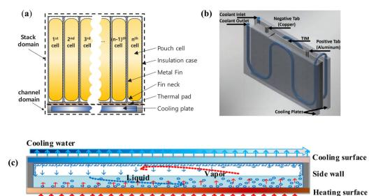
Fig. 12 (a) Typical structure of battery stack with metal fin and cooling plate, <sup>144</sup> (b) the geometry of the proposed liquid-based TMS, <sup>145</sup> (c) schematic of the longitudinal section of the vapor chamber. 146
