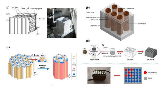
Fig. 16 (a) Battery pack and cooling structure, <sup>169</sup> (b) structure of the battery pack simulation set, <sup>170</sup> (c) battery module consisting of multiple 21700 cells and simplified CAD model for the module,  $^{171}$  and (d) manufacture of CSG and configuration of detected batteries.  $^{173}$
