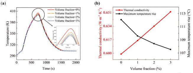
Fig. 9 Effect of nanoparticle volume fraction on the novel BTMS: (a) temperature change under different nanoparticle volume fractions;<sup>129</sup> (b) thermal conductivity and maximum temperature rise under different nanoparticle volume fractions.<sup>129</sup>
