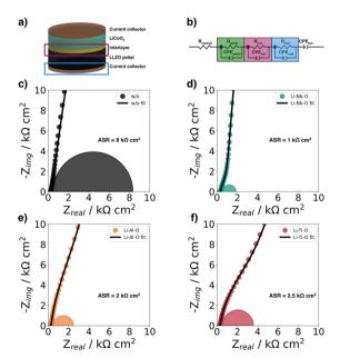
Fig. 5 (a) Schematic of half-cells structure for electrochemical impedance spectroscopy at room-temperature, (b) equivalent circuit model used to fit the impedance spectra by Zhang et al., 43 EIS spectra of (c) Au|LCO|LLZO|Au (w/o), (d) Au|LCO|Li-Nb-O|LLZO|Au (Li-Nb-O), (e) Au|LCO|Li-Al-O|LLZO|Au (Li-Al-O), and f) Au|LCO|Li-Ti-O|LLZO|Au (Li-Ti-O). The measured data are shown together with the fits from the equivalent circuit
