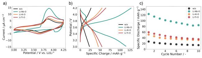
Fig. 6 (a) Cyclic voltammetry scans measured with a sampling rate of  $0.1 \text{ mV s}^{-1}$  between 3 and 4.25 V vs. Li/Li<sup>+</sup>, (b) charge–discharge curves with 1.75  $\mu$ A cm<sup>-2</sup> between 3 V and 4.2 V at 80 °C, and (c) specific discharge capacities for full cells with and without interface modification.
