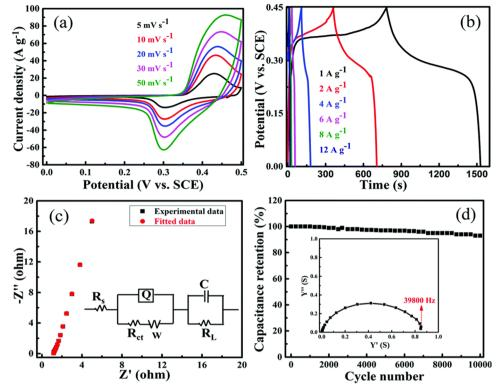
Fig. 12 Electrochemical responses of 10 PGNC composite (a-d) CV curves at different scan rates, GCD at different applied current densities, Impedance plot, cycling stability at 8 A g<sup>-1</sup> with admittance plot. Reproduced with permission, <sup>92</sup> Copyright (2020), Royal Society of Chemistry.
