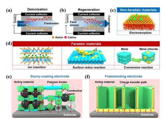
Fig. 1 Schematic illustration of the (a) deionization process, (b) regeneration process, ion uptake mechanisms of (c) non-Faradaic materials and (d) Faradaic materials, and specific features of a (e) slurry-coating electrode and (f) freestanding electrode.
