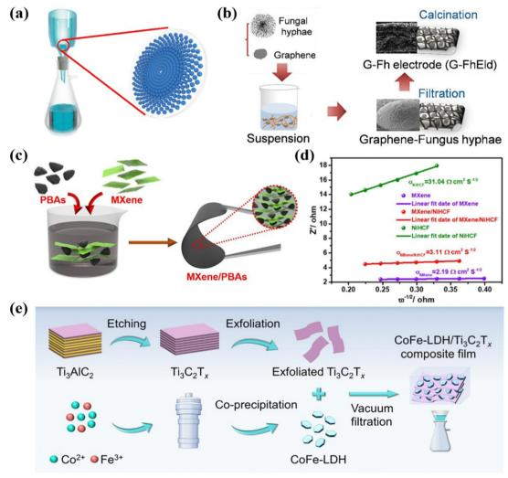
Fig. 4 (a) Schematic illustration of vacuum filtration. Schematic diagram of (b) preparation of a graphene-fungus hyphae electrode, (c) fabrication and (d) Z' vs. frequency ( $\omega^{-1/2}$ ) of the freestanding MXene/Prussian blue analogues electrodes, and (e) CoFe-LDH/MXene synthesis. Reproduced from ref. 105 and 113 with permission from Elsevier, and reproduced from ref. 112 with permission from American Chemical Society.
