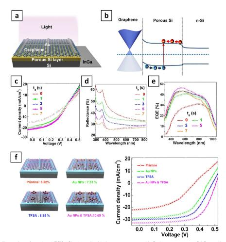
Fig. 13 (a) Schematic illustration of graphene/PSi/n-Si solar cell with Au top contact and InGa bottom contact. (b) Energy band diagrams of the device. (c)–(e) J-V characteristics, reflectance, and EQE spectra of the devices with  $t_d$  from 0 to 7 s. (f) J-V characteristics, and (d) EQE spectra of the pristine, individually doped (Au NPs or TFSA), and co-doped graphene layers/PSi solar cells. Reproduced from ref. 163, with permission from the Royal Society of Chemistry.
