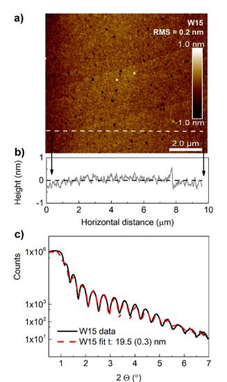
Fig. 1 (a) AFM image for a typical W film. (b) Surface roughness profile. (c) Low angle X-ray data and the fitting for a W15 thin film.
