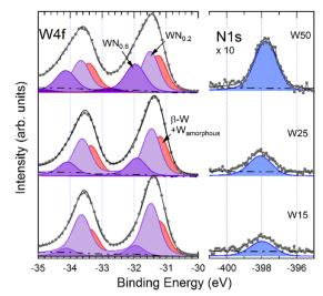
Fig. 6 W4f and N1s spectra for W thin film growth in reactive gas mixtures with N<sub>2</sub> (%): 15, 25, and 50. With the progressive incorporation of nitrogen, we identified different tungsten nitride phases:  $\sim WN_{0.2}$  and  $\sim WN_{0.6}$ .
