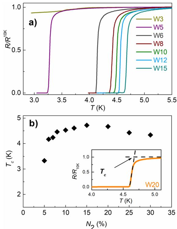
Fig. 3 (a) Temperature dependence of the normalized resistivity for films grown for 1 minute using different reactive Ar/N<sub>2</sub> atmospheres (thickness between 18 and 20 nm). (b) Summary of the superconducting critical temperature as a function of the N<sub>2</sub> concentration in the reactive gas mixture.
