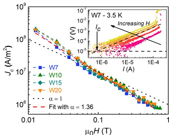
Fig. 7 Magnetic field dependence of the critical current density,  $J_c$ , for films grown for 1 minute (thickness between 18 and 20 nm). The measurements were performed with the magnetic field perpendicular to the surface of the films. Inset: Typical IV curves in log-log scales and the criterion for the determination of  $J_c$ .
