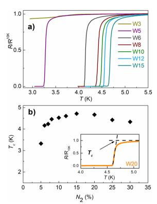
Fig. 3 (a) Temperature dependence of the normalized resistivity for films grown for 1 minute using different reactive Ar/N<sub>2</sub> atmospheres (thickness between 18 and 20 nm). (b) Summary of the superconducting critical temperature as a function of the N2 concentration in the reactive gas mixture.
