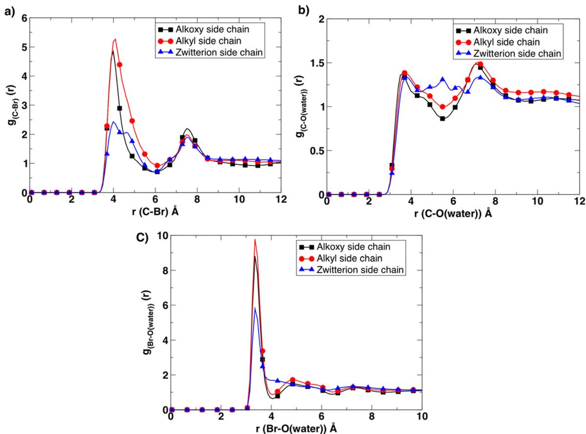
Fig. 4 The radial distribution function  $g(r)$  between (a) the C atom (the first methylene group of the side chain attached to the pyridinium N atom) and the bromide atom. (b) The C atom (the first methylene group of the side chain attached to the pyridinium N atom) and water O atom. (c) The radial distribution function  $g(r)$  calculated between the bromide atom and water O atom.
