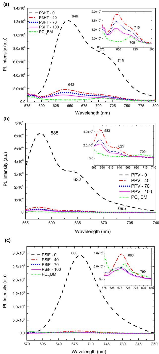
Fig. 4 Photoluminescence (PL) emission spectra of (a) P3HT, (b) MDMO-PPV and (c) PSiF-DBT for pure conjugated polymer nanoparticles, pure fullerene PC<sub>71</sub>BM nanoparticles and polymer/PC<sub>71</sub>BM heterojunction nanoparticles with fullerene doping amount of 40%, 70% and 100%. The inset in PL spectra shows the emission intensity for samples of fullerene doping amount of 40%, 70%, 100% and PC<sub>71</sub>BM nanoparticles.
