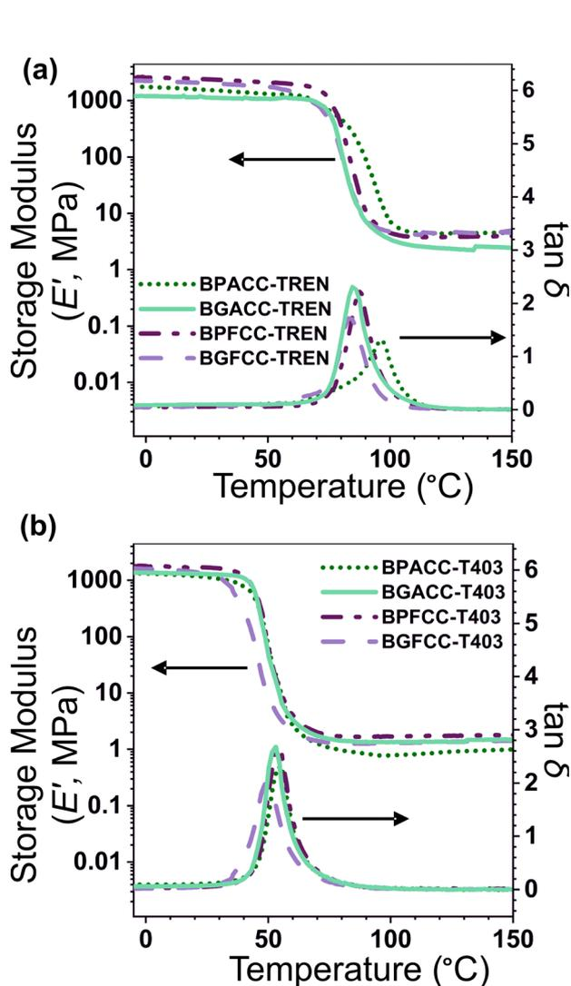
Fig. 3 Storage modulus and  $\tan \delta$  as a function of temperature for (a) TREN-based and (b) T403-based NIPU networks. Data shown are from the second heating cycle of DMA experiments, in oscillatory film tension mode at a heating rate of 3 °C min<sup>-1</sup>, strain amplitude of 0.3%, frequency of 0.1 Hz, and an axial force of 0.4 N.
