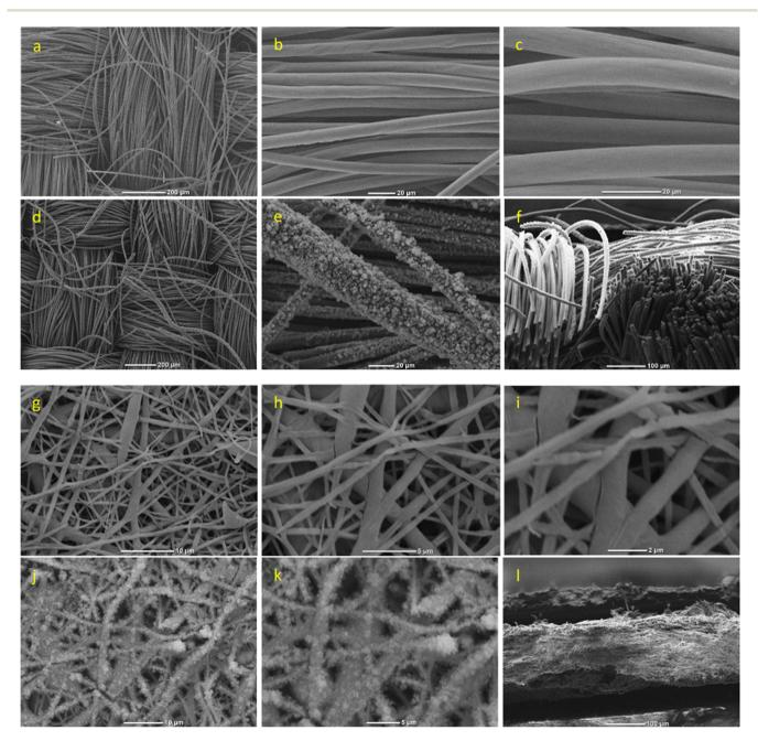
Fig. 3 SEM images of: (a-c) the uncoated carbon cloth (CC). (d and e) EDOT-co-EDOTSAc-co-EDOTEG coated CC. (f) Cross section of EDOT-co-EDOTSAc-co-EDOTEG coated CC. (q-i) uncoated electrospun fibers (EF). (j and k) EDOT-co-EDOTSAc-co-EDOTEG coated EF, (l) cross-section of EDOT-co-EDOTSAc-co-EDOTEG coated EF.
