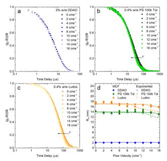
Fig. 7 (a) DLS correlograms obtained for a solution of 3% w/w DDAO in water as a function of flow velocity (0–16 cm s $^{-1}$ ) in a 1 mm ID glass capillary. (b) *idem* for 0.4% w/w PS 100k in toluene, (c) *idem* for 0.4% w/w Ludox AS 40 in water. (d) Apparent  $R_{\rm H}$  extracted from the velocity-dependent model (solid lines and symbols); for comparison, results from a simple exponential decay (dashed lines and open symbols) are included.
