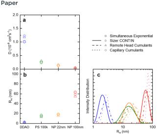
Fig. 3 (a) Translational diffusion coefficients D, (b) mean hydrodynamic radii  $R_{\rm H}$ , and (c) size distributions obtained for DDAO micelles, PS (100k) polymer chains in solution, ludox NP 22 nm, and polystyrene latex 100 nm. These results are obtained from the raw data shown in Fig. 2.
