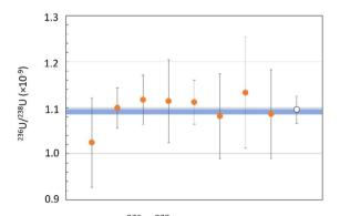
Fig. 3 Measurement of <sup>236</sup>U/<sup>238</sup>U isotope ratios in IRMM 075/6 certified reference material. The open dot corresponds to the mean of the measurements (red dots). The blue rectangle highlights the certified value uncertainties. Uncertainties are extended with a coverage factor of 2.
