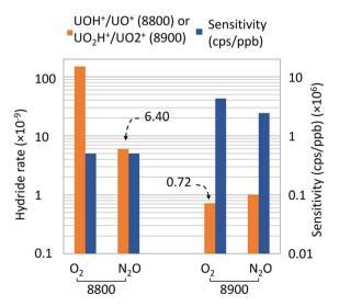
Fig. 2 Comparison of the hydride formation rate and sensitivity with Agilent 8800 ICP-MS/MS (left) from Jaegler et al. (2020) and Agilent 8900 ICP-MS/MS (right) using O<sub>2</sub> or N<sub>2</sub>O as a reaction gas in the CRC.
