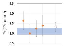
Fig. 6 Measurements of <sup>236</sup>U/<sup>238</sup>U isotope ratios in MTG sample. The open dot corresponds to the mean of the measurements (red dots). The blue rectangle highlights the certified value uncertainties. Uncertainties are extended with a coverage factor of 2.
