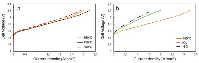
Fig. 6 Comparison of *I–V* curves at 60 °C (a) among the differently treated NiFeOx-based cells and (b) among the cells equipped with NiFe-oxide 450, IrO<sub>2</sub>, and NiO at the anode.
