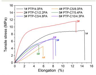
Fig. 5 Stress-strain curves of the PTP and PTP-Cx membranes doped in 85 wt% PA solution at  $60 \, ^{\circ}$ C.
