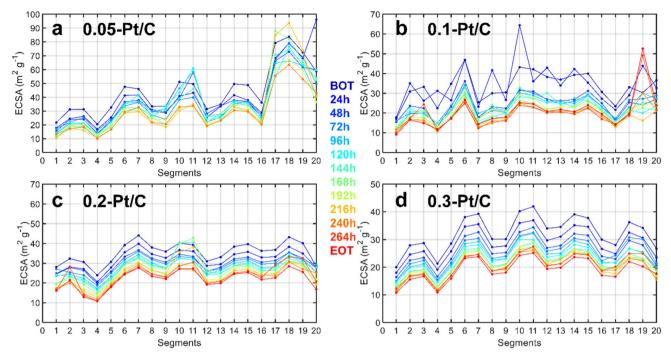
Fig. 3 Local ECSA along the gas channel measured in a segmented cell for CLs (a) 0.05-Pt/C; (b) 0.1-Pt/C; (c) 0.2-Pt/C and (d) 0.3-Pt/C. Segment #1 corresponds to the air inlet at the cathode and  $H_2$  outlet at the anode, while segment #20 corresponds to the air outlet at the cathode and  $H_2$ inlet at the anode.
