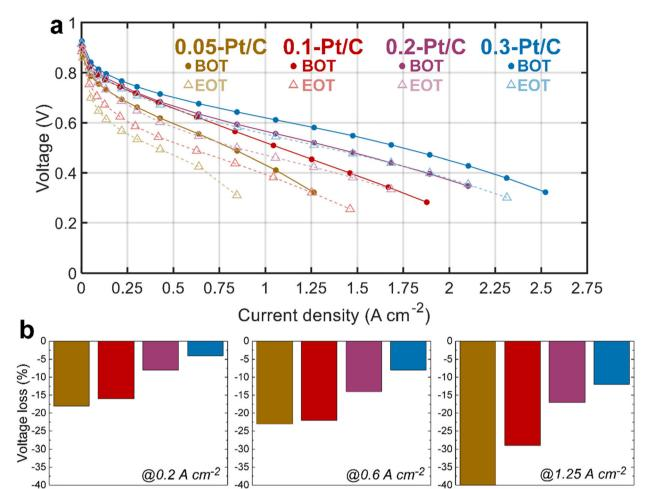
Fig. 1 (a) Polarization curves for the MEAs comprising 0.05-Pt/C, 0.1-Pt/C, 0.2-Pt/C and 0.3-Pt/C cathode CLs at BOT and EOT; (b) voltage losses of selected points at low (0.2 A cm<sup>-2</sup>), medium (0.6 A cm<sup>-2</sup>) and high (1.25 A cm<sup>-2</sup>) current densities.
