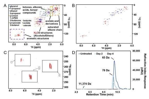
Fig. 3 <sup>1</sup>H-<sup>13</sup>C HSQC NMR spectra of (A) untreated PHW; (B) PHW after 5 days of MEC treatment. Note that the edited HSQC shows CH<sub>2</sub> in blue and CH/CH<sub>3</sub> in red. (C) <sup>1</sup>H-<sup>15</sup>N HMBC NMR spectrum of untreated PHW, with the insets showing enlarged view of each peak. (D) Size-exclusion chromatography of PHW at different stages of MEC treatment.
