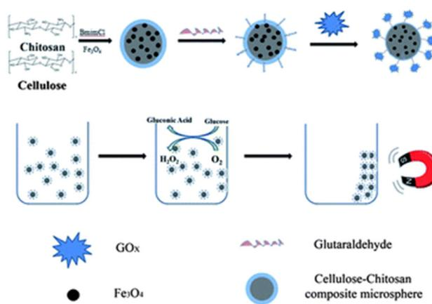
Fig. 17 Preparation of magnetic Fe<sub>3</sub>O<sub>4</sub>-cellulose-chitosan microspheres after enzyme immobilization onto magnetic cellulose-chitosan (schematic). Reproduced from ref. 79 with permission from RSC, copyright 2012.
