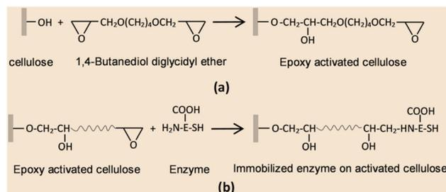
**Fig. 10** Plausible reaction mechanism of enzyme immobilization through the epoxy method. (a) Surface reaction of a cellulose matrix with 1,4-butanediol diglycidyl ether (BTDE). (b) Covalent coupling of enzyme onto the surface of activated cellulose. Reproduced from ref. 54 with permission from Elsevier, copyright 2018.
