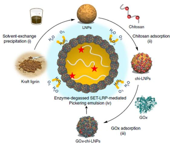
**Fig. 12** Preparation of GOx-chi-LNPs and application in enzyme-degassed SET-LRP-mediated Pickering emulsion (Schematic). (i) Preparation of LNPs via solvent-exchange precipitation. (ii) Adsorption of chitosan on LNPs to yield chi-LNPs. (iii) Adsorption of GOx on chi-LNPs to yield GOx-chi-LNPs. (iv) Application of GOx-chi-LNPs as biocatalytic degassing stabilizers for SET-LRP in Pickering emulsion media. Reproduced from ref. 92 with permission from Nature Portfolio, copyright 2020.
