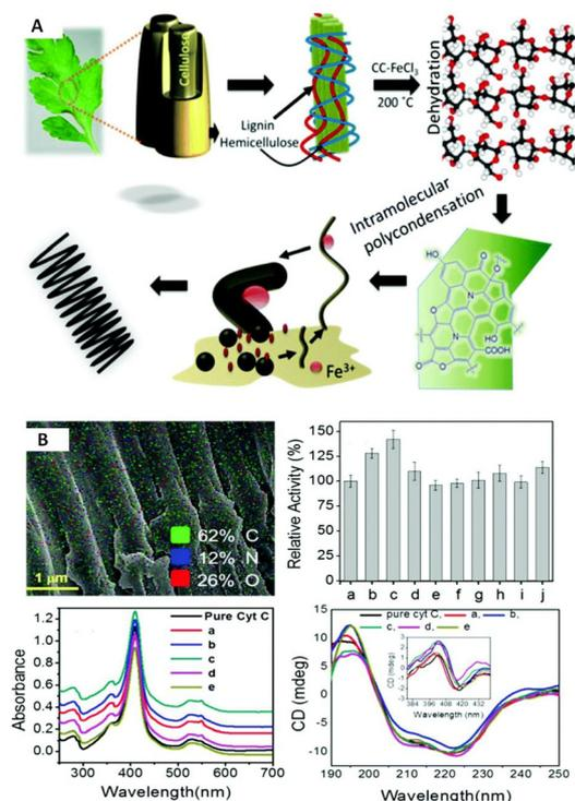
**Fig. 9** Schematic depictions of (A) a plausible mechanism of the sequential growth of TLFCs from *Parthenium* biomass during a solvo-thermal process in the presence of a DES (CC : FeCl<sub>3</sub>, 1 : 2 mol ratio) (B) Cyt C immobilized on TLECH and showing activity and stability results (ref. 50).
