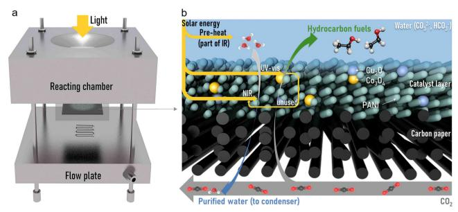
Fig. 1 (a) The assembly of the bifunctional gas diffusion system. (b) Energy and mass flow in the GDL.
