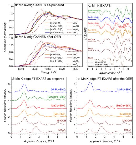
Fig. 2 Mn K-edge (a and b) XANES, (c) EXAFS and (d and e) FT EXAFS data collected for the [Mn + Sb]O<sub>x</sub> (orange), [MnCo + Sb]O<sub>x</sub> (red), [MnPb + Sb]O<sub>x</sub> (blue) and [MnCoPb + Sb]O<sub>x</sub> (green) catalysts before and after OER tests (10 mA cm<sup>-2</sup>, 24 h, 24  $\pm$  2 °C) compared to relevant reference materials (see figure). In panel c, dashed and solid traces show data collected before and after the OER tests, respectively.
