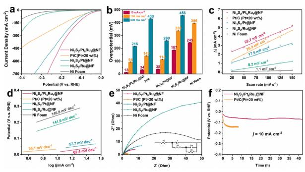
Fig. 2 Electrocatalytic HER performance in 1.0 M KOH solution. (a) Polarization curves of the electrocatalysts for the HER (with 95% iR compensation), (b) the resultant overpotentials at current densities of 10, 100 and 500 mA cm $^{-2}$  for the as-prepared electrocatalysts, (c) calculated electrochemical double-layer capacitances, (d) the corresponding Tafel plots, (e) Nyquist plots under open-circuit voltage, and (f) long-term stability test at current densities of 10 mA cm $^{-2}$ .
