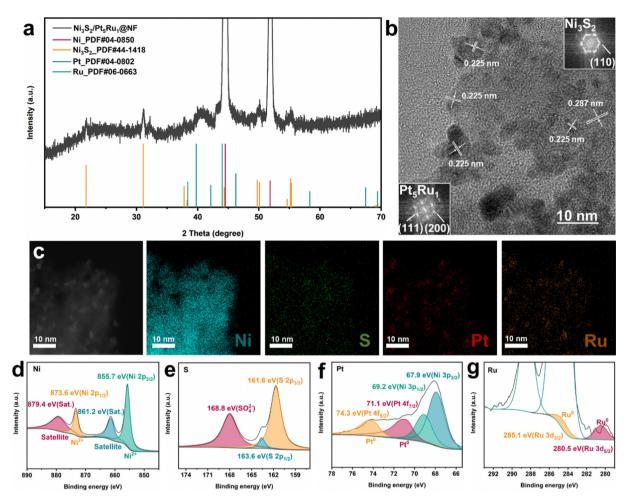
Fig. 1 Structural and microstructure characterizations of Ni<sub>3</sub>S<sub>2</sub>/Pt<sub>5</sub>Ru<sub>1</sub>@NF. (a) XRD pattern, (b) HRTEM image and the corresponding FFT patterns, (c) STEM image and the corresponding EDX elemental mapping images, and XPS spectra of (d) Ni 2p, (e) S 2p, (f) Pt 4f, and (g) Ru 3d.
