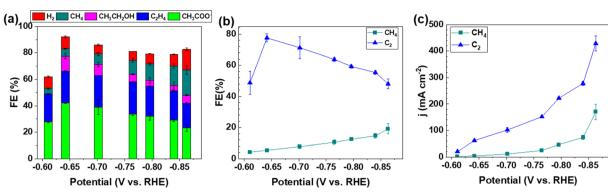
Fig. 1 (a) Product distribution during the CORR as a function of the applied potential on the CP-Cu<sub>0.812</sub> electrode. (b) FEs of C<sub>2</sub> and CH<sub>4</sub>. (c) The partial current density of C2 and CH4. The error bars represent the standard deviation from the measurements of three independent electrodes.
