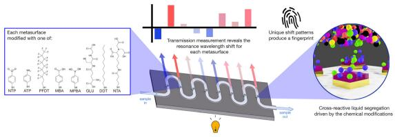
Fig. 1 Schematic of the sensor concept. Eight metasurfaces are linked by a microfluidic channel. Each metasurface is modified with a different surface chemistry, providing partial-selectivity to the components in the water sample. Thus, each metasurface experiences a unique refractive-index environment, shifting its resonance wavelength value. By tracking the combination of resonance shifts we build a fingerprint for each sample.
