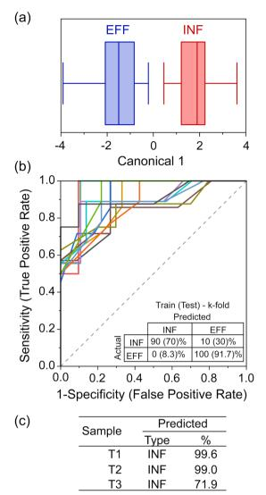
Fig. 4 (a) LDA of the sensor response (input is average resonance shift from DI water per NTB per sample, with k-fold cross validation, k = 5) comparing INF and EFF groups, only. (b) ROC curves and (inset) the averaged (25 iterations) classification table for the accuracy of the training set and the validation set. (c) The predicted classification and percent probability for the three excluded tap water samples, using the LDA model.
