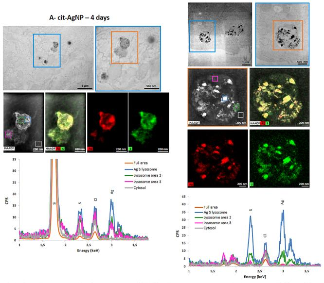
Fig. 4 AgNP transformations in vesicles. Chemical analysis by STEM-EDX of spheroid sections exposed for 4 days to cit-AgNP (A) or to PVP-AgNP (B). STEM micrograph field of view showing the presence of vesicles containing transformed AgNP (upper panels). EDX maps of the vesicle located in the orange box (middle panels). EDX spectra of the different regions selected in the HAADF map (colored boxes) in the energy range 1-3.5 keV (lower panels). The position of Si, S, Cl and Ag peaks is highlighted.
