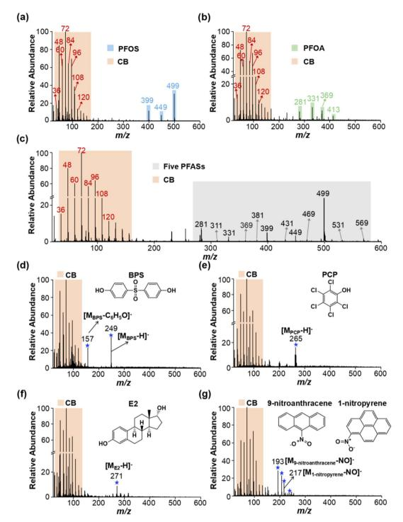
Fig. 1 Simultaneous analysis of EC and multiple types of OCs by LDI-MS. The typical MS spectra of (a) PFOS, (b) PFOA, (c) five PFASs, (d) BPS, (e) PCP, (f) E2, and (g) 9-nitroanthracene and 1-nitropyrene mixed with CB standard. *Note*: CB was a model EC. PFASs (including PFOS, PFOA, PFNA, PFDA and PFDoA), BPS, PCP, E2, 9-nitroanthracene, and 1-nitropyrene were used as representative OCs. The detailed information about these characteristic peaks is listed in Table S1.†
