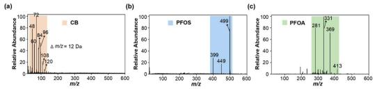
The mass spectra of individual standards of (a) CB ( $0.1 \text{ mg mL}^{-1}$ ), (b) PFOS (100 ng mL $^{-1}$ ), and (c) PFOA (100 ng mL $^{-1}$ ) obtained by LDI-MS.
