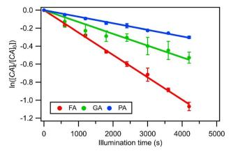
Fig. 2 Photodegradations of FA, GA, and PA in nitrate-mediated photooxidation experiments using 250  $\mu$ M AN at pH 4. Error bars represent standard deviations of repeated measurements. Lines show the exponential fit to the photodegradation data.
