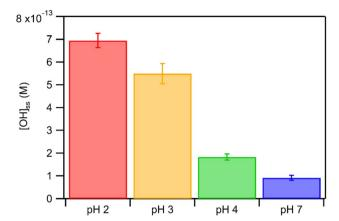
Fig. 4 Estimated [·OH]<sub>ss</sub> in nitrate-mediated photooxidation experiments using 250  $\mu M$  AN at pH 2, 3, 4, and 7. Error bars represent standard deviations of multiple experiments.
