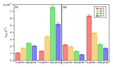
Fig. 3  $k_{obs}$  of FA and GA at pH 2, 3, 4, and 7. The concentrations of FA and GA were fixed at 10  $\mu$ M, while either 250  $\mu$ M or 1250  $\mu$ M AN were used in these experiments. Error bars indicate standard deviation of multiple experiments.
