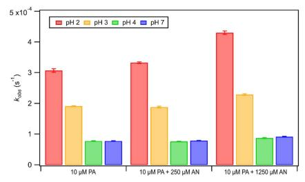
Fig. 6  $k_{obs}$  of PA at pH 2, 3, 4, and 7. The PA concentration was fixed at 10 μM, while either 0 μM or 250 μM or 1250 μM AN were used in these experiments. Error bars indicate the standard deviation of multiple experiments.
