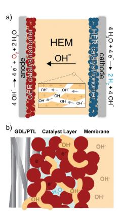
Fig. 1 Ion transport and reactivity in HEM electrolyzers. Schematics of (a) electrolyzer cell and (b) anode-catalyst layer. The OH- anions conduct through the ionomer, and electrons conduct through the catalyst. Oxygen evolution occurs at the ionomer/catalyst interface.
