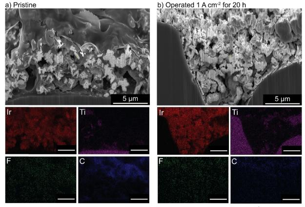
Fig. 5 Cross-sectional imaging and EDX of an  $IrO_x/20\%$  TP-85 anode PTE. (a) Before and (b) after 20 h operation at 1 A cm<sup>-2</sup>. All scale bars are 5  $\mu$ m. No ionomer is observed in the catalyst layer after operation.
