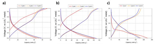
Fig. 8 Voltage profiles for BM-Li<sub>2</sub>MoO<sub>4</sub> using varying voltage ranges: (a) 4.8-2.0 V, (b) 4.8-1.5 and (c) 3.0-1.0 V. Note: cell c was discharged first before charging to higher voltages.
