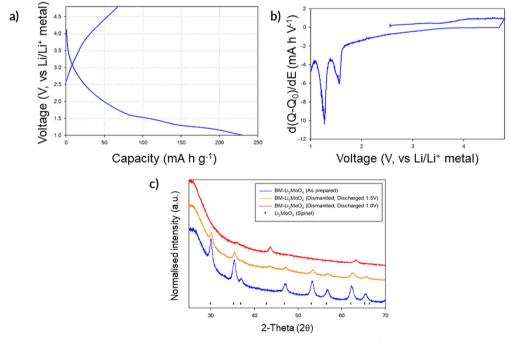
Fig. 7 (a) First cycle voltage profile for BM-Li<sub>2</sub>MoO<sub>4</sub> cycled in the region of 4.8-1.0 V at 10 mA  $g^{-1}$ ; (b) associated dQ/dV plot of the first charge/discharge cycle; (c) PXRD of dismantled swagelok cells showing phases formed once discharged down to 1.5 and 1.0 V (Cu K $\alpha$ ).
