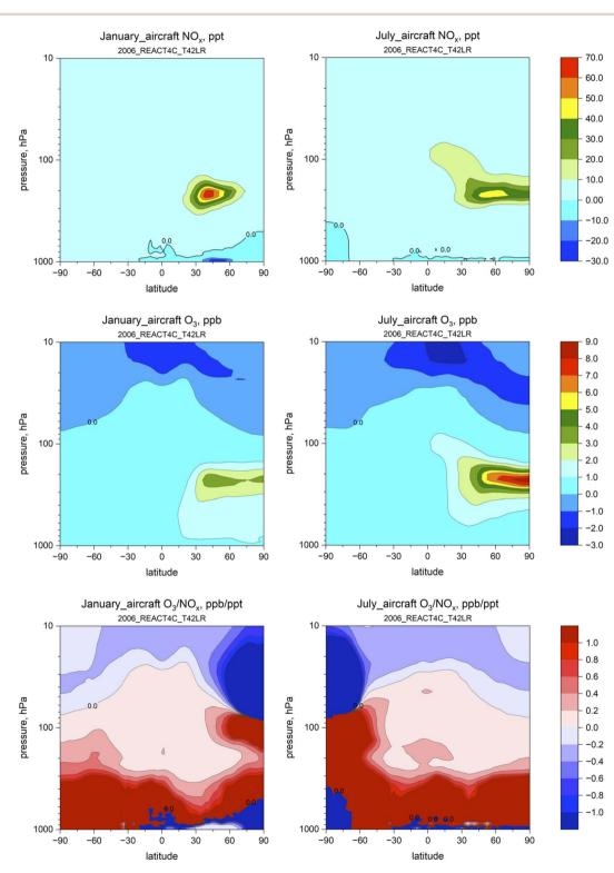
Fig. 10 Two-dimensional (latitude by height) averaged  $NO_x$  concentrations (VMR – volume mixing ratios) from aircraft (upper panels, left–right, Jan and July) in ppt, the resultant ozone concentration perturbations (middle panels) and the sensitivity of ozone to  $NO_x$  (ozone ppb/ $NO_x$  ppt). Data from Skowron *et al.* (2015)<sup>69</sup> simulations.
