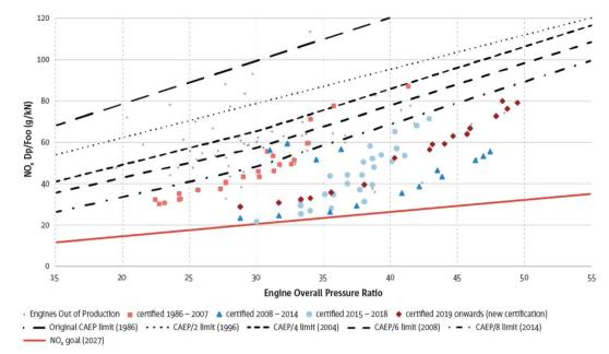
Fig. 2 Engine  $NO_x$  emissions certification data<sup>39</sup> showing the metric as ordinate and the pressure ratio as abscissa. The lines represent the various CAEP standards and goals.
