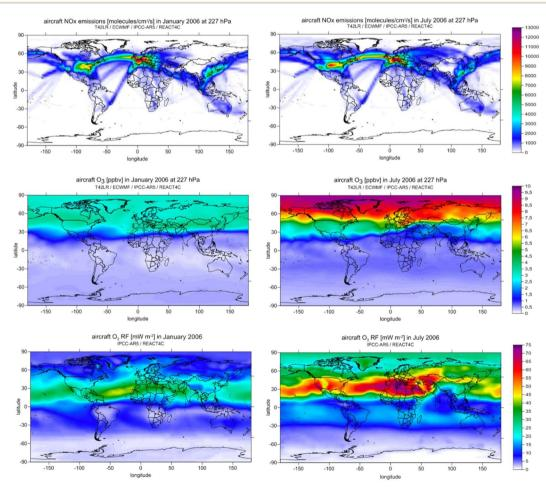
Fig. 9 Simulations of global aircraft NO<sub>x</sub> emissions in 2006, January (upper left-hand panel), July (upper right-hand panel), ozone concentrations attributable to the aircraft NO<sub>x</sub> at 227 hPa (approximately 11 km) (middle panels) in ppb, and the consequential radiative forcing (lower panels) (data replotted from simulations described by Skowron et al., 2015). 69
