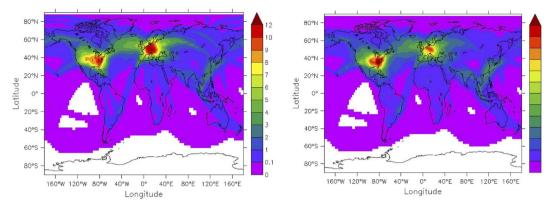
Fig. 8 Model simulation of the global distribution of contrail cirrus coverage associated with a visible optical thickness ≥0.05 in percent (left hand panel) and the net radiative forcing due to contrail cirrus in mW m<sup>-2</sup> (right hand panel). Taken from Fig. 5 of Bier and Burkhardt (2022).<sup>61</sup>
