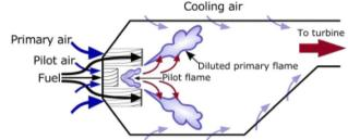
Fig. 3 Sketches of combustion chambers from Bergthorson and Thomson (2015),<sup>40</sup> showing RQL (top) and TAPS lean burn (bottom) combustors.
