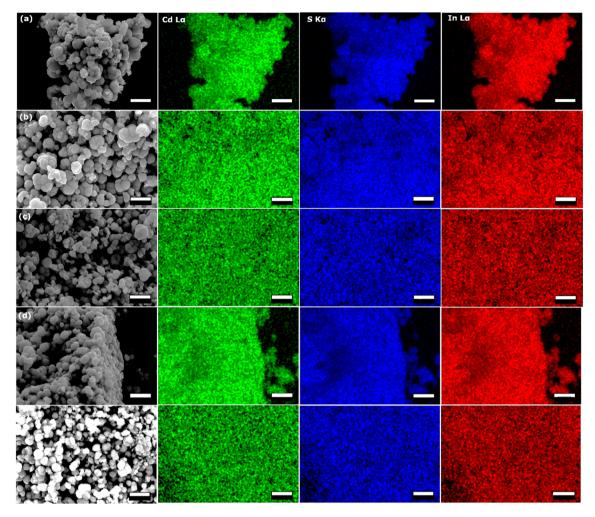
Fig. 7 EDX spectroscopic mapping (20 keV) of Cd L $\alpha$ , In L $\alpha$  and S K $\alpha$  for In $_x$ Cd $_{1-x}$ S $_{1+0.5x}$  samples. (a) x=0.02, (b) x=0.04, (c) x=0.06, (d) x=0.08 and (e) x=0.1 mole fractions of gallium. All scale bars correspond to 5  $\mu$ m.
