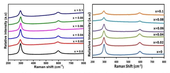
Fig. 8 Raman spectra of (lhs)  $Ga_xCd_{1-x}S_{1+0.5x}$ , where x = 0, 0.02, 0.04, 0.06, 0.08 and 0.1 and (rhs)  $In_xCd_{1-x}S_{1+0.5x}$ , where x = 0, 0.02, 0.04, 0.06, 0.08 and 0.1.
