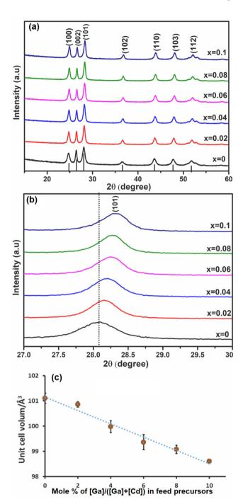
Fig. 2 (a) p-XRD patterns of Ga-doped CdS with different mole fractions of  $Ga_xCd_{1-x}S_{1+0.5x}$ ,  $0 \le x \le 0.1$ ; (b) an expanded view of (101) plane diffraction for  $Ga_xCd_{1-x}S_{1+0.5x}$  and (c) unit cell volume Å<sup>3</sup> of nanoparticles of  $Ga_xCd_{1-x}S_{1+0.5x}$  as a function of Ga mol% where mol% is defined as a % of total metals content *i.e.* [Ga]/([Cd] + [Ga])%.
