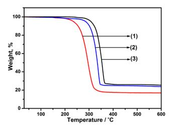
Fig. 1 Thermogravimetric analysis (TGA) profiles of (1)  $[Ga(DTC)_3]$  (expected for  $Ga_2S_3$ : 22.9%), (2)  $[Cd(DTC)_2]$  (expected for CdS: 25.5%) and (3)  $[In(DTC)_3]$  (expected for  $In_2S_3$ ; 29.1%).
