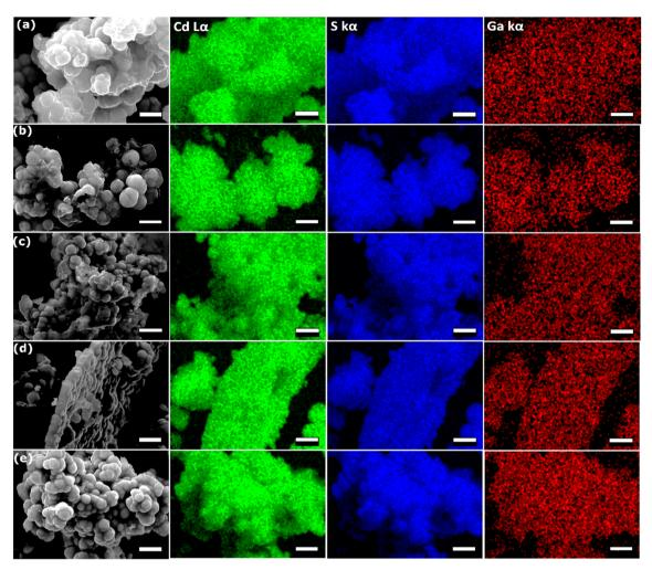
Fig. 4 EDX spectroscopic mapping (20 keV) of Cd L $\alpha$ , Ga L $\alpha$  and S K $\alpha$  for Ga<sub>x</sub>Cd<sub>1-x</sub>S<sub>1+0.5x</sub> samples. (a) x = 0.02, (b) x = 0.04, (c) x = 0.06, (d) x = 0.08and (e) x = 0.1 mole fractions of gallium. All scale bars correspond to 5  $\mu$ m.
