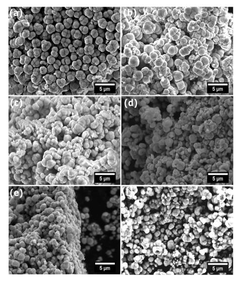
Fig. 6 SEM images (10 keV) of doped and undoped samples of  $\ln_x Cd_{1-x}S_{1+0.5x}$ , x = 0 (a), x = 0.02 (b), x = 0.04 (c), x = 0.06 (d), x = 0.08 (e) and x = 0.10 (f).
