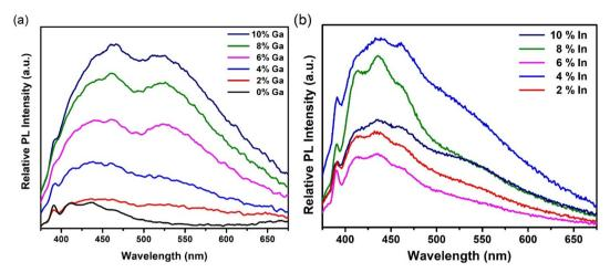
Fig. 9 (a) PL spectra of undoped and Ga-doped CdS nanoparticles (b) PL spectra of In-doped CdS nanoparticles at an excitation wavelength of 350 nm.
