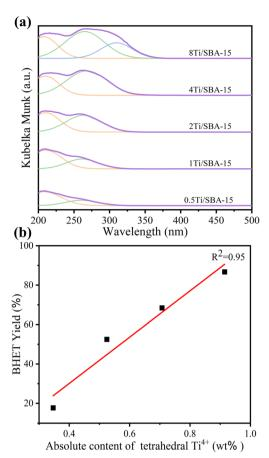
Fig. 9 (a) DR UV-vis spectra of Ti/SBA-15 with different Ti loadings. (b) The linear relationship between the absolute content of tetrahedral Ti<sup>4+</sup> species and the BHET yield.
