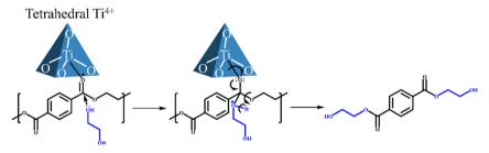
Scheme 2 Reaction mechanism of PET glycolysis catalyzed by Ti/SBA-15
