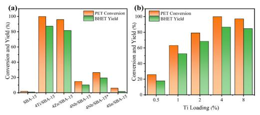
Fig. 1 (a) BHET yield obtained over different catalysts. Reaction conditions: 0.4 g PET, 2.8 g EG, 50 mg catalyst, 1 MPa N<sub>2</sub>, 190 °C, 45 min. "\*" means the reaction time is 2 h. (b) Influence of Ti loadings on BHET yield. Reaction conditions: 0.4 g PET, 2.8 g EG, 20 mg catalyst, 1 MPa N<sub>2</sub>, 190 °C, 45 min.
