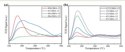
Fig. 2 (a) NH<sub>3</sub>-TPD curves of various M/SBA-15 catalysts and (b) Ti/SBA-15 with different Ti loadings.
