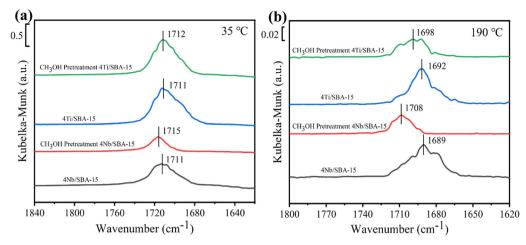
Fig. 5 Acetone DRIFTS spectra of 4Nb/SBA-15, 4Nb/SBA-15 pretreated with methanol, 4Ti/SBA-15, and 4Ti/SBA-15 pretreated with methanol recorded at (a) 35 °C and (b) 190 °C, respectively.
