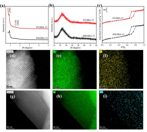
Fig. 3 (a) Small- and (b) wide-angle XRD patterns of 4Nb/SBA-15 and 4Ti/SBA-15. (c) N2 adsorption-desorption isotherms of 4Nb/SBA-15 and 4Ti/ SBA-15. (d) HADDF-STEM image of 4Ti/SBA-15. (e and f) EDS mapping images of Si (e) and Ti (f) in 4Ti/SBA-15. (g) HADDF-STEM image of 4Nb/ SBA-15. (h and i) EDS mapping images of Si (h) and Nb (i) in 4Nb/SBA-15.
