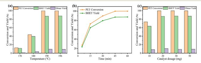
Fig. 6 (a) Influence of reaction temperature on PET conversion and BHET yield. Reaction conditions: 0.4 g PET, 2.8 g EG, 50 mg 4Ti/SBA-15, 1 MPa N<sub>2</sub>, 45 min. (b) Reaction time curves of PET glycolysis. Reaction conditions: 0.4 g PET, 2.8 g EG, 50 mg 4Ti/SBA-15, 1 MPa N<sub>2</sub>, 190 °C. (c) Influence of catalyst dosage on PET conversion and BHET yield. Reaction conditions: 0.4 g PET, 2.8 g EG, 1 MPa N<sub>2</sub>, 190 °C, 45 min.
