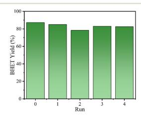
Fig. 8 The reusability of 4Ti/SBA-15 in the glycolysis of PET. Reaction conditions: 0.4 g PET, 2.8 g EG, 30 mg 4Ti/SBA-15, 1 MPa N2, 196 °C,
