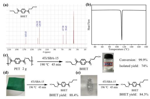
Fig. 7 (a) 13C NMR spectrum and (b) DSC curve of BHET obtained from PET glycolysis. (c) The flow chart of PET glycolysis scale-up experiment. (d and e) The flow charts of common real PET plastics glycolysis.
