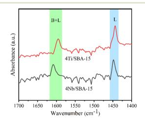
Fig. 4 FT-IR spectra of pyridine adsorbed on 4Nb/SBA-15 and 4Ti/ SBA-15 recorded at 200 °C.
