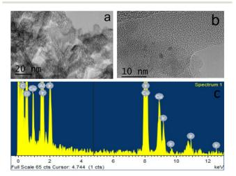
Fig. 9 A and B. HRTEM images of  $3@Al_2O_3$ -uncal after 45 h reaction at 350 °C with 0.10 mL min<sup>-1</sup> flow rate. A few particles, 2–3 nm in diameter are visible at higher magnification. The lattice spacing corresponds to metallic Ir. C. XEDS spectra of  $3@Al_2O_3$ -uncal after 45 h reaction.
