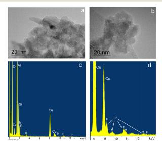
Fig. 3 HRTEM images and XEDS spectra of 3@Al<sub>2</sub>O<sub>3</sub>-uncal (a and c) and of 3@Al<sub>2</sub>O<sub>3</sub>-cal (b and d). The full spectrum is shown in c) and expanded around the Ir-family L-peaks in d. The Cu peaks are from the sample grid.
