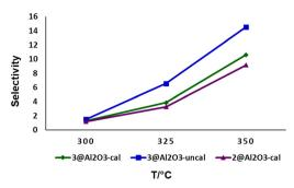
Fig. 6 Selectivity for P3 at different temperatures using various catalysts (selectivity =  $[P3/(P1 + P2 + P3)] \times 100$ ), flow rate = 0.09 mL min<sup>-1</sup>.
