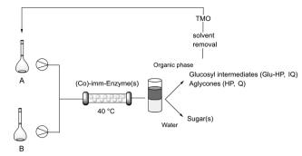
Scheme 2 Flow bioprocessing of HES and RT. Solution A: 10 g L<sup>-1</sup> HES or RT in TMO. Solution B: HEPES buffer, 0.05 M, pH 7.5. Co-immenzyme(s): imm-RN (5 mg  $g_{resin}^{-1}$ ) or HOR (1 mg  $g_{resin}^{-1}$ ) or imm-RN-HOR (5 mg<sub>RN</sub> g<sub>resin</sub><sup>-1</sup>, 1 mg<sub>HOR</sub> g<sub>resin</sub><sup>-1</sup>). T = 40 °C.
