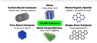
Fig. 4 Various types of CO<sub>2</sub>RR catalysts.
