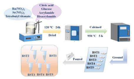
Fig. 1 The synthesis process of BST photocatalysts.
