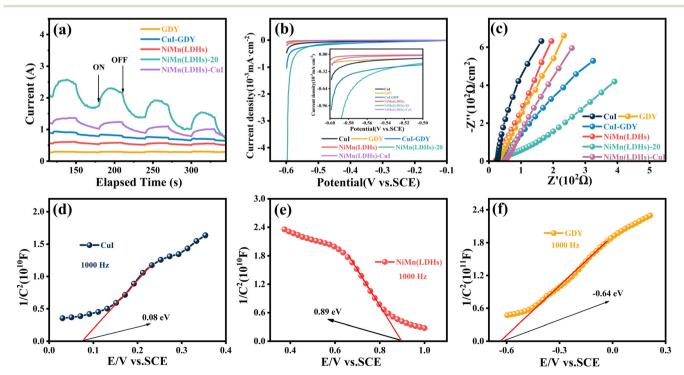
Fig. 10 (a) Transient photocurrent response of GDY, Cul-GDY, NiMn(LDHs), NiMn(LDHs)-Cul, NiMn(LDHs)-20; (b) LSV curves and (c) EIS spectra of Cul, GDY, Cul-GDY, NiMn(LDHs), NiMn(LDHs)-Cul, NiMn(LDHs)-20; (d-f) Mott-Schottky plots of Cul, NiMn(LDHs), and GDY.
