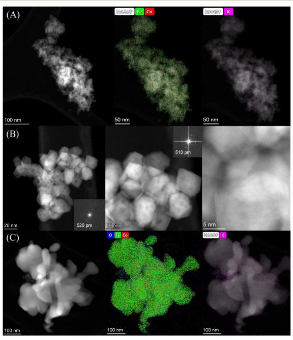
Fig. 1 HAADF-STEM images and corresponding elemental mapping images of the Fe<sub>9</sub>CoK<sub>6</sub> catalyst (A and B) before reduction and (C) after reduction. The insets in B show the FFT patterns.
