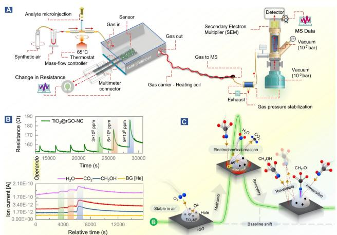
Fig. 5 Room temperature methanol gas sensing on 50% TiO<sub>2</sub>@rGO-NC monitored by operando mass spectrometry (MS). (A) Experimental design of operando-resistance/mass spectroscopy of the surface electrochemical reaction upon methanol gas exposure, (B) change in resistance due to the methanol stimulus with simultaneous detection of product molecules, and (C) illustration of the methanol sensing mechanism; see text for details
