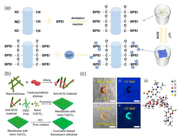
Fig. 13 The sensing and removal mechanism of functional polymer membranes for heavy metal ions in. (a) The preparation of aPAN/BPEI NMs and detection/removal of Cu<sup>2+</sup>. Reproduced from ref. 107 with permission from American Chemical Society. Copyright 2021. (b) The preparation of anti-ACQ materials. (c) The optical image of CAM under natural light and ultraviolet light and the optical image of anti-ACQ material under natural light and ultraviolet light.
