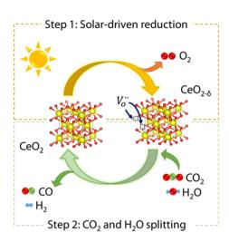
Fig. 2 Scheme of the thermochemical cycle for CO<sub>2</sub> and H<sub>2</sub>O splitting over CeO<sub>2</sub>. Reproduced with permission from ref. 26 with permission from RSC
