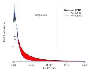
Fig. 4 KERDs for m/z 202 recorded at the lowest (7.5 eV) and highest (12.0 eV) photon energy. Assuming that the former belongs only to parent monomer ions, the amount of dissociative ionisation contributing to the m/z 202 channel can be estimated by previous subtraction (after normalisation using the area delimited by N) of the "cold" KERD. The percentage of fragmentation is then given by the red area, divided over the total distribution.
