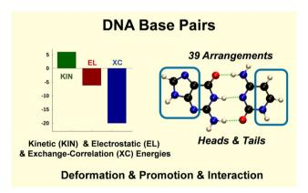
Fig. 9 IQA contributions to the bond energy for the G···C base-pairing interaction. Geometries and electron densities were computed for 39 different base pairs and their corresponding individual bases at the M06-2X/TZVP computational level. Reprinted with permission from ref. 200 Copyright 2021 American Chemical Society.
