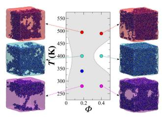
Fig. 13 Temperature-volume fraction ( $\Phi$ ) phase diagram for polystyrene  $(M_W = 4800) + n$ -hexane. The snapshots correspond to equilibrium configurations of the system at different temperatures. Greyed-out regions correspond to the two-phase regions. Dashed lines are smoothed experimental data. Taken with permission from ref. 205. Copyright 2017 American Chemical Society.
