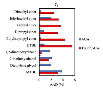
Fig. 5 Comparison of the average absolute deviations of the AUA and TraPPE-UA force fields for the prediction of boiling point data for ethers and glycols. Boiling point calculations differed against DIPPR data by no more than 5% for TraPPE-UA and no more than 4% for AUA. Adapted with permission from ref. 113. Copyright 2013 Taylor & Francis.
