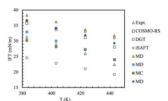
Fig. 9 Benchmark and predicted interfacial tensions for the water/50:50 n-dodecane + toluene mixture. The uncertainty is of the order of 1 mN m<sup>-1</sup> for the experimental data and aprox. 0.5-3 mN m $^{-1}$  for the predictive methods. Adapted with permission from ref. 77. See original source for the full discussion of the methods and force-fields used. Copyright 2018 Elsevier.
