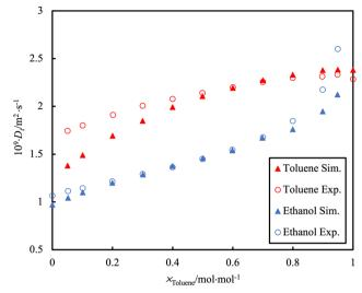
Fig. 8 PFG-NMR data (open symbols) for the self-diffusion, D, of individual toluene or ethanol molecules in the binary mixture at 298.15 K and ambient pressure as compared to simulation data (filled symbols). Adapted with permission from ref. 171. Copyright 2018 Springer Nature.
