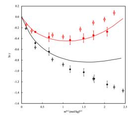
Fig. 6 Mean ionic activity coefficient,  $\gamma$ , of NaCl in water at (red) 298.15 K and 1 bar and (black) 473.15 K and 15.5 bar *versus* molality, *m*. Solid lines are experimental data. Filled symbols are polarizable models, open symbols are fixed charge models. Adapted with permission from ref. 149. Copyright 2015 American Chemical Society.
