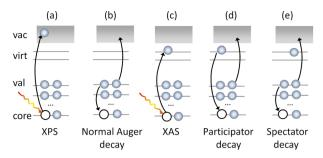
Fig. 1 Schematic pictures of studied X-ray spectroscopies. (a) XPS – X-ray photoelectron spectroscopy, (b) AES - normal (non-resonant) Auger electron spectroscopy (2h), (c) XAS - X-ray absorption spectroscopy and possible follow-up decay mechanisms (d) participator decay (1h) and (e) spectator decay (2h1p).
