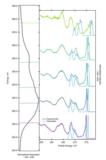
Resonant Auger spectra. The left panel shows the XAS spectrum, the lines show energies at which the resonant Auger spectra were measured: 285.02, 285.32, 285.56, 285.94, 286.54 eV. The right panel shows individual resonant Auger spectra. Light blue line corresponds to the calculations at the EOM-CC/cc-pVTZ level for a set of structures with appropriate electronic transition energies (within 90 meV range)
