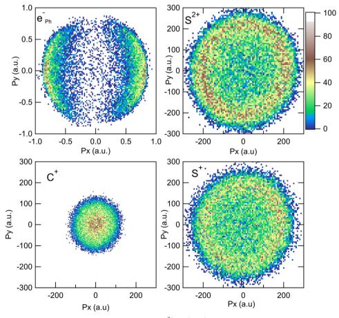
Fig. 1 Momentum distributions recorded in the laboratory frame for the  $S^{2+} + C^+ + S^+ + e_{ph}^-$  PE3PICO channel after core S 1s photoionization in CS<sub>2</sub>.
