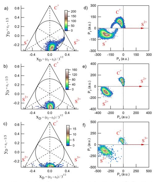
Fig. 3 Dalitz diagrams and Newton plots obtained for the three main three-body dissociation channels (see Table 1 for details) after core S 1s photoionization in CS2. The Dalitz diagrams for channels (2), (4) and (7) are represented in subplots a, b, and c, respectively. The corresponding Newton plots are represented in subplots d, e, and f.
