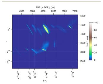
Fig. 2 Three-ion coincidence map recorded in PE3PICO measurements after core S 1s photoionization in CS<sub>2</sub>
