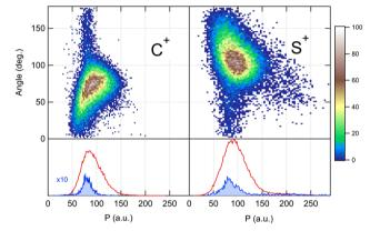
Fig. 7 Angular dependence of the momentum distributions measured for the two fragment ions C<sup>+</sup> and S<sup>+</sup> produced in the dissociation of CS<sup>2+</sup> in the second step of the dissociation of the molecular ion CS<sub>2</sub><sup>4+</sup>. Bottom panels show the 1D projection of the total momentum distributions in red and for selected angular ranges in solid blue. See the text for details.
