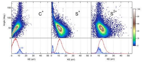
Fig. 6 Angular dependence of the kinetic energy distributions measured for the three fragment ions produced in the dissociation of CS<sup>4+</sup> after core S 1s photoionization in CS<sub>2</sub>. Bottom panels show the 1D projection of the total kinetic energy distributions in red, and the partial distributions in solid blue for a selected range of angles (see the text for details).
