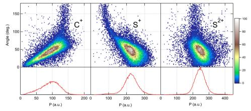
Fig. 5 Angular dependence of the momentum distributions measured for the three fragment ions produced in the dissociation of CS<sup>4+</sup> after core S 1s photoionization in CS2. Bottom panels show the 1D projection of the total momentum distributions.
